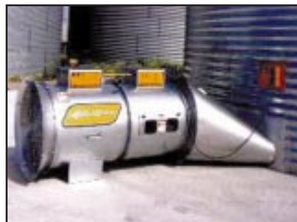
Figure 15.2. Typical centrifugal fan with heater and controls on an on-farm bin.
